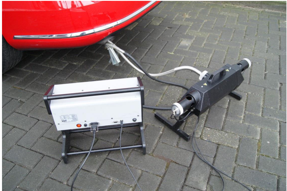
Figure 4 Opacity was measured using two types of opacity or smoke meters. The conventional EDA2 (right), and the modern, more accurate LPA (left). Both smoke meters are manufactured by TEN Automotive Equipment. As the picture shows, the in-line opacity meters were inserted into the exhaust pipe simultaneously.
