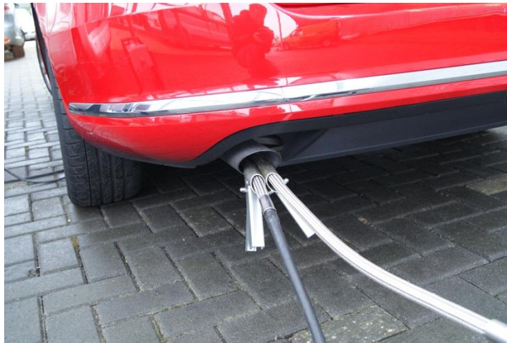
Figure 9 The probes of the LPA and EDA2 opacity meters were both inserted into the tailpipe during the free acceleration test and the high idle speed test. This way, both smoke meters measured simultaneously. Also see Figure 4.
