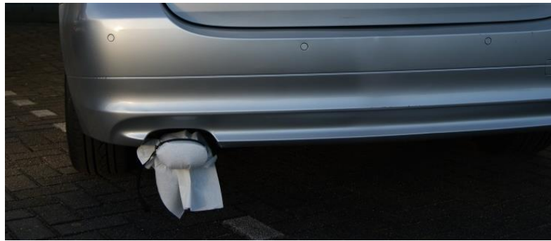
Figure 16 In the tissue filter test, a tissue was attached to the end of the exhaust pipe after which the engine was let running at idle speed for three minutes. Cars showing elevated emissions in previous tests were selected for the TFT.
