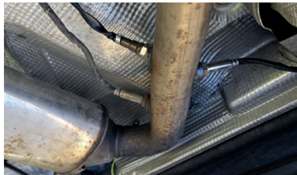
The SEMS system includes one or two NO x sensors and an NH 3 sensor, which can be easily attached to the exhaust of a vehicle.
