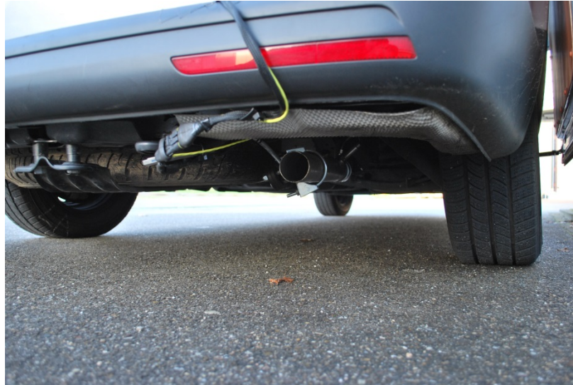
Figure 3: \text{NO}_x sensor and thermocouple mounted in the vehicle's tailpipe.
