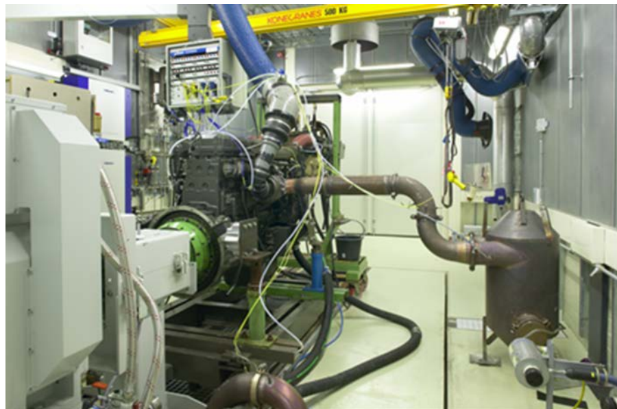
Figure 2: engine test bed for heavy duty testing.
